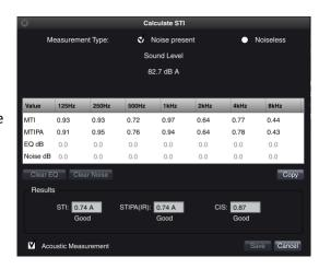
Acquiring a suitable impulse response measurement, choosing the correct measurement type for the system under test, and providing accurate input parameters requires a thorough understanding of the STI standard to achieve trustworthy results. The Smaart v8 User Guide will be updated to include a comprehensive section explaining STI and the measurement process.
